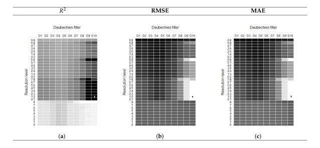
**Figure 4.** Goodness of fit metrics for the best wavelet transfer function models fitted to DANC: (a) Coefficient of determination ( $\mathbb{R}^2$ ). Maximum values are identified (Max in D10, resolution 1:2). (b) Root mean squared error (RMSE). Minimum values are identified (Min in D10, resolution 1:2). (c) Mean absolute error (MAE). Minimum values are identified (Min in D10, Resolution 1:2).
