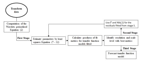
Figure 1. Process diagram for transfer function model with time varying coefficients.
