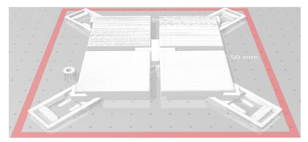
**Figure 3.** Illustration of the exemplary obtained STL model of four 3D scanned samples with visible mounting elements.
