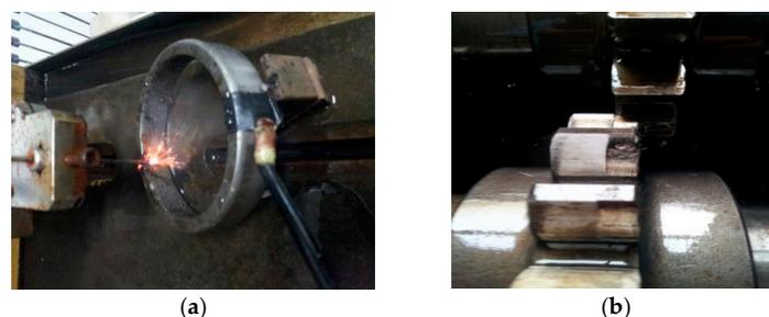
Figure 16. Bearing and gear fault diagram. (a) Bearing outer ring defect; (b) Gear peeling.
