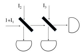
**Figure 2.** A classical photon analog encounters two beamsplitters, and is divided among three detectors. The CPA is boosted by some unknown peak intensity  $I_1$ , and each beamsplitter's dark port has an additional incident field with unknown intensity.
