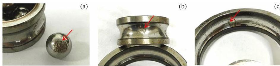
Figure 9. Tested bearing with different fault types: (a) roller fault, (b) inner race-way fault, and (c) outer race-way fault.
