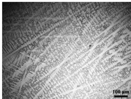
**Figure 1.** Optical micrograph of the as-cast NiCrFeCoMn alloy.
