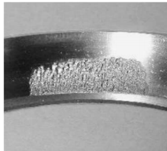
Figure 13. Photo of outer race defect in bearing 1 after the test.
