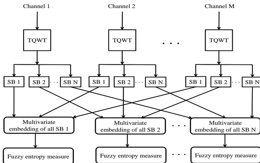
**Figure 1.** TQWT based multivariate sub-band fuzzy entropy.
