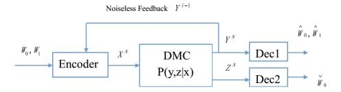
Figure 1. Broadcast channel with confidential messages and noiseless feedback.
