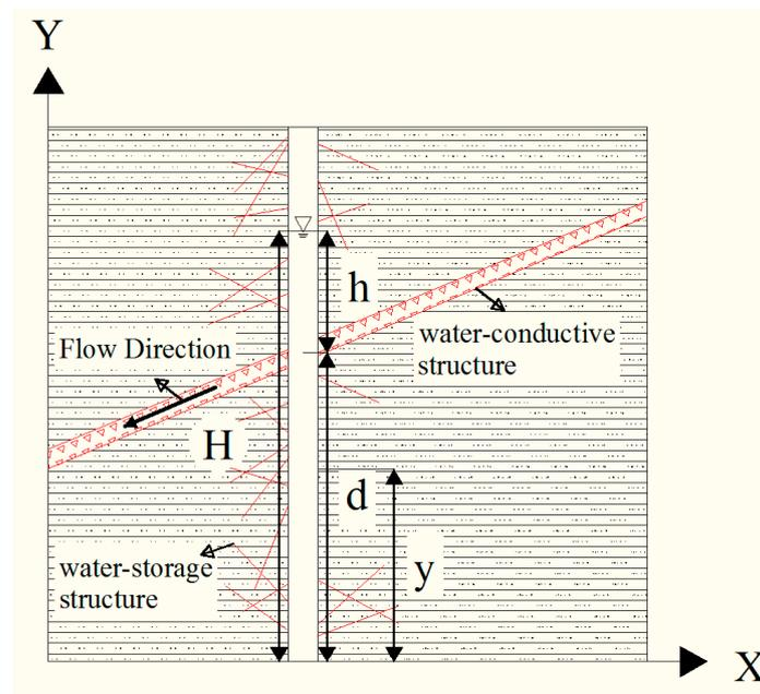
Figure 1. Model diagram of seepage velocity in a borehole.
