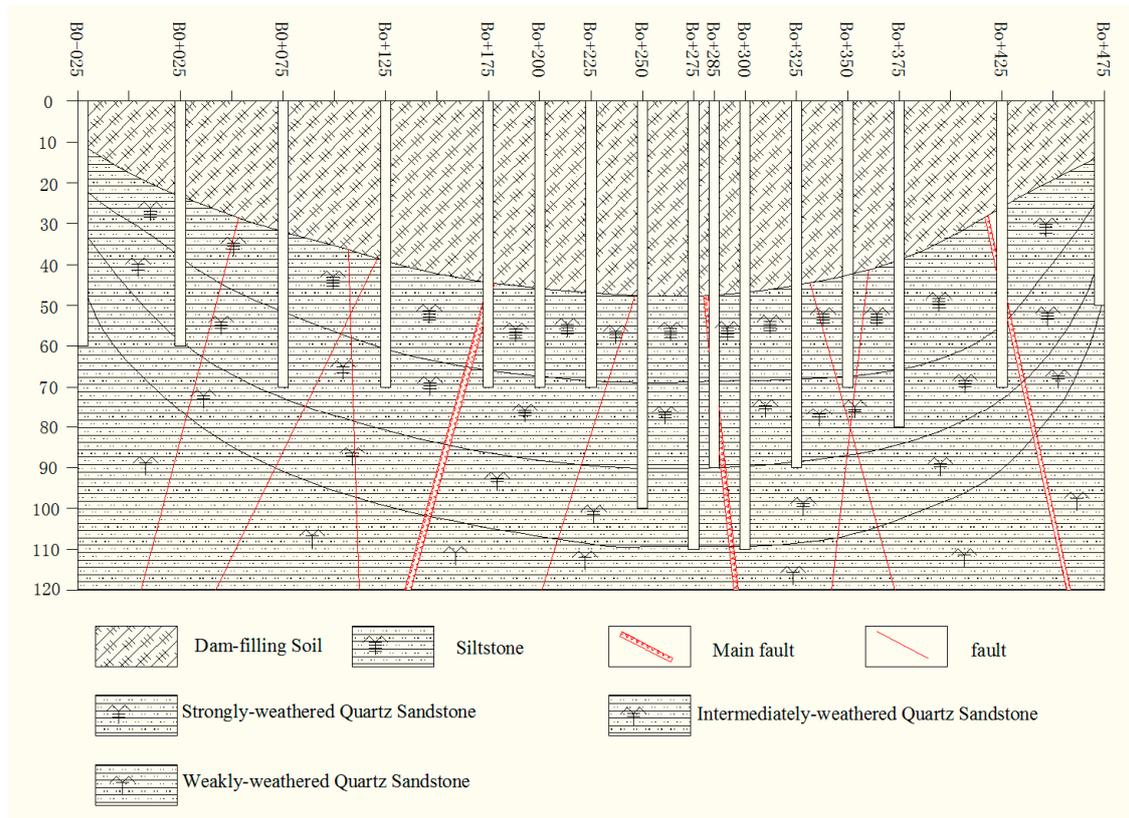
Figure 2. Cross-section geological map of the dam site.
