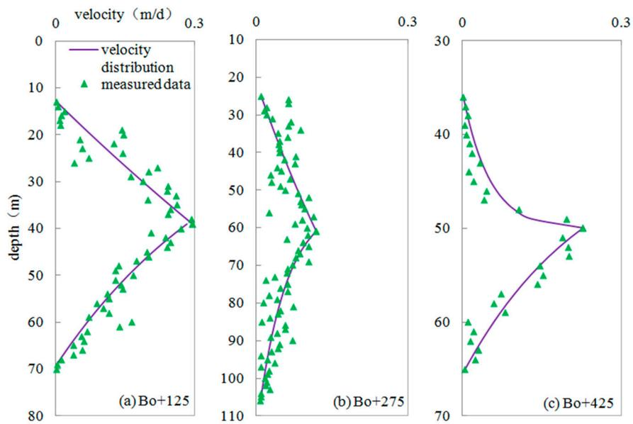
**Figure 3.** Comparison between the computed seepage velocity distribution and the measured data in (a) Bo+125, (b) Bo+275, and (c) Bo+425.
