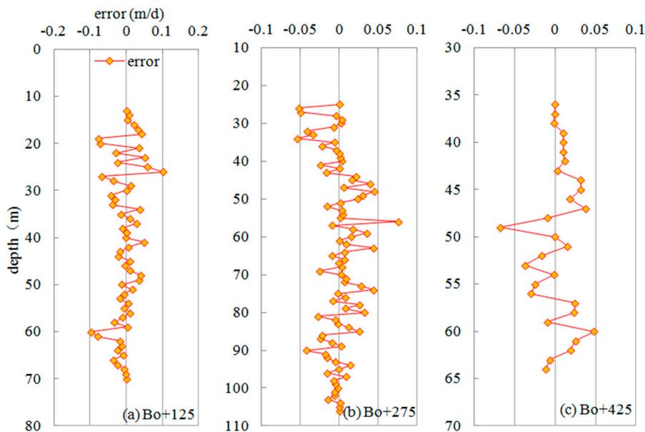
**Figure 4.** Deviation of the computed seepage velocity distribution from the measured data at each measured point in (a) Bo+125, (b) Bo+275, and (c) Bo+425.
