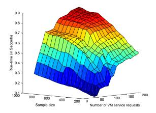
Figure 3. Run-time of CEVMAC on a 3.20-GHz i5-3470 CPU from Intel for different experimental settings.
