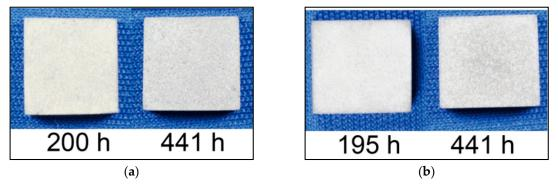
**Figure S1.** The isothermal oxidation resistance of the Al<sub>0.2</sub>Co<sub>1.5</sub>CrFeNi<sub>1.5</sub>Ti<sub>0.3</sub> alloy after aluminizing: the surface morphology samples at (a) 1173 K for 200 h and 441 h; and (b) 1273 K for 195 h and 441 h.
