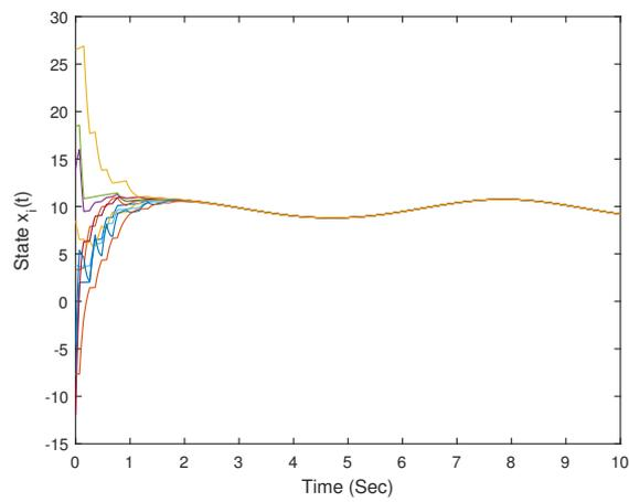
Figure 5. State  $x_i(t)$  under the state-controlled switching topologies without a threshold.
