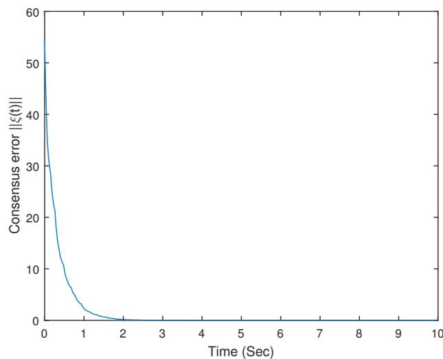
Figure 7. Consensus error  $\|\xi(t)\|$  under the state-controlled switching topologies without a threshold.
