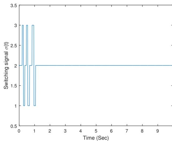
**Figure 3.** The state-controlled switching signal  $\sigma(t)$  with a threshold  $\varpi = 0.1$ .
