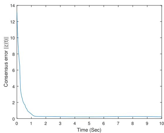
**Figure 4.** Consensus error  $\|\tilde{\xi}(t)\|$  under the state-controlled switching topologies with a threshold  $\varpi = 0.1$ .
