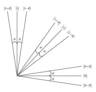
**Figure 2.** Collective-rotation model on qubit states  $|1\rangle$ ,  $|x\rangle$  and  $|0\rangle$ .
