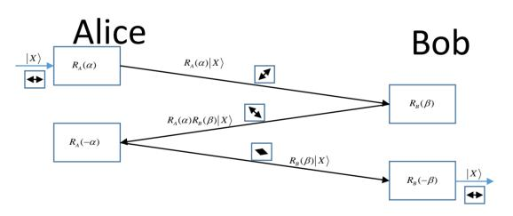
Figure 1. Schematic diagram of the three-stage protocol.
