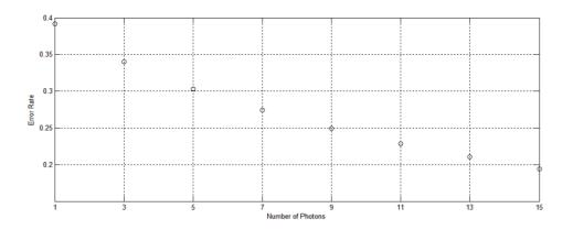
Figure 6. Error rate versus number of photons when deflection angle is 15°.
