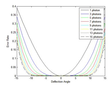
Figure 3. Error rate versus deflection angle in multi-photon system with odd numbers.
