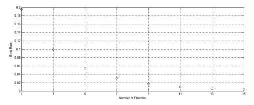
Figure 5. Error rate *versus* number of photons when deflection angle is 10°.
