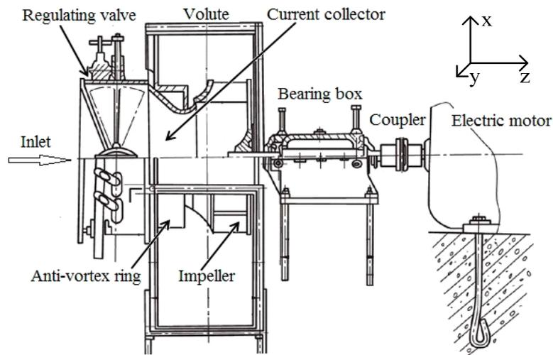
Figure 2. Geometrical model of the centrifugal fan.
