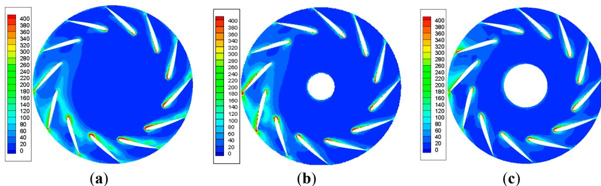
3.5. Entropy Generation Characteristics During the Circumference Propagation of Stall Cell
