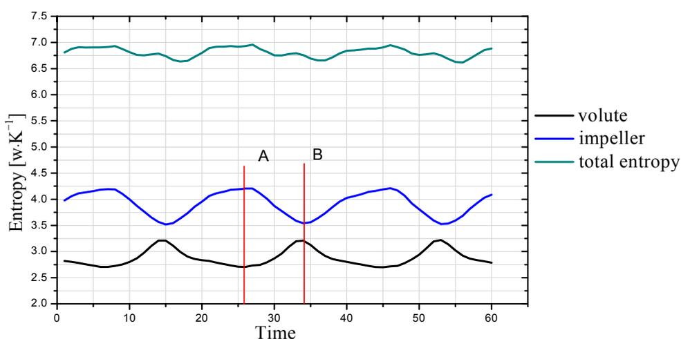
The average entropy generation of the impeller is  $3.866 \text{ w}\cdot\text{K}^{-1}$ , and the amplitude is  $0.338 \text{ w}\cdot\text{K}^{-1}$ . The average entropy generation of the volute is  $2.959 \text{ w}\cdot\text{K}^{-1}$ , and the amplitude is  $0.254 \text{ w}\cdot\text{K}^{-1}$ . The
