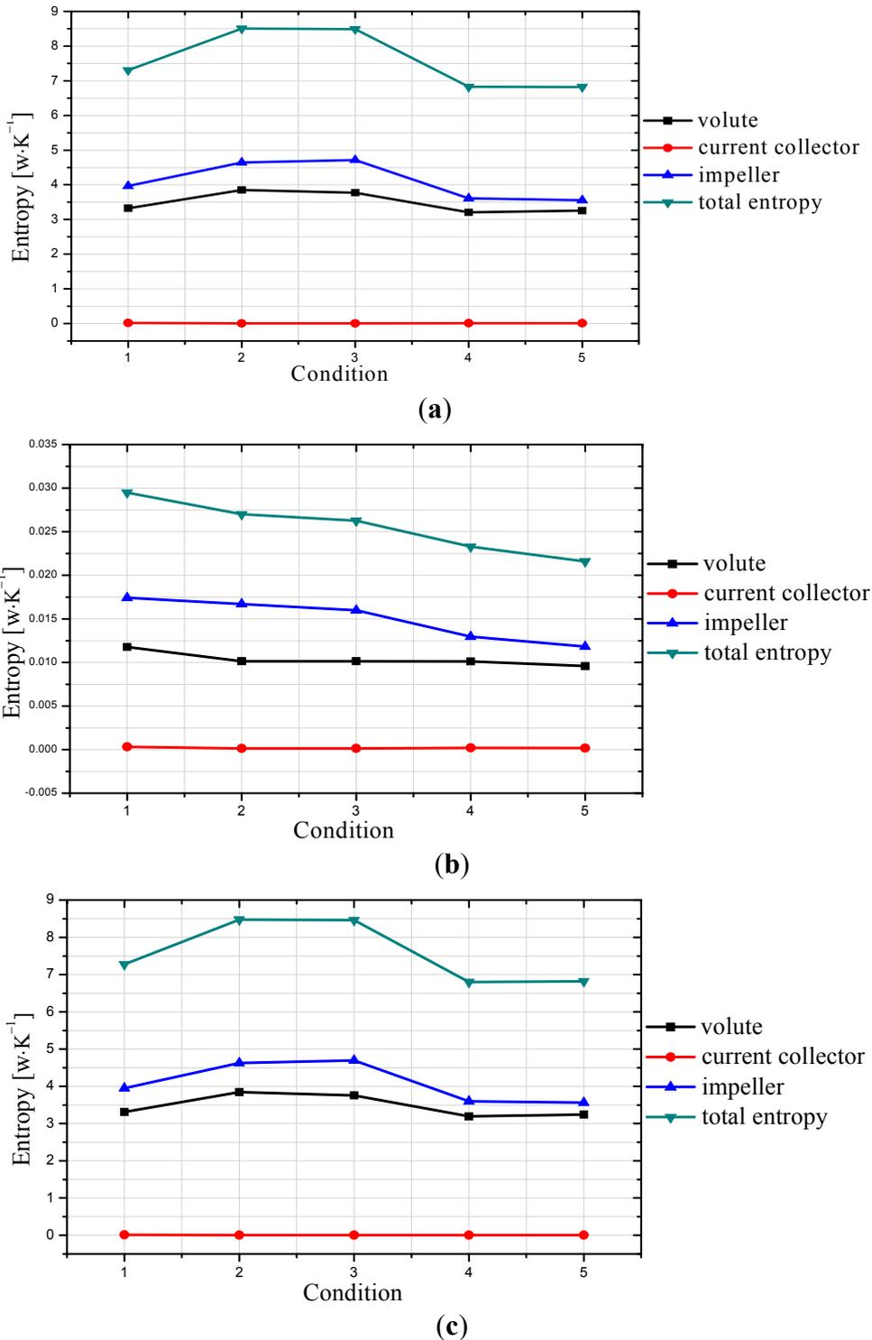
Comparing Figure 8b with Figure 8c, the entropy generation caused by viscous dissipation is very small and it is two orders of magnitude lower than the entropy generation caused by turbulence dissipation. Therefore, the energy loss of the fan mainly comes from the turbulent dissipation, while the viscous dissipation can nearly be ignored.
