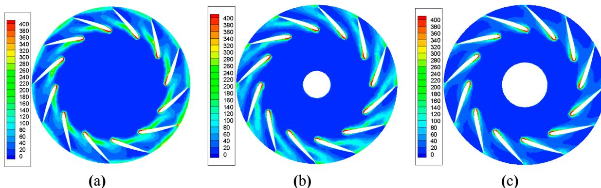
Figure 11 shows the contours of entropy generation on the three cross sections mentioned above in the 185th revolution. The distribution of the entropy generation is non-uniform on  $z = 31$  cm section. There are two high entropy generation areas and one of them is near the volute tongue.
