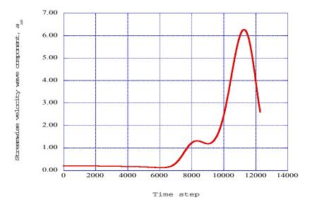
Figure 3 presents the streamwise velocity wave component the normal velocity wave component at the fifth streamwise station (x = 0.16). These results indicate that as the normal velocity wave component increases, the streamwise velocity component decreases. This indicates an outward "*ejection*" of flow that approaches a near vertical configuration.
