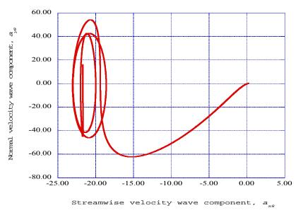
Figure 7 shows the phase plane,  $a_{z8}$ - $a_{y8}$ , for the output at streamwise station eight. These results indicate an oscillatory motion in the normal-spanwise plane, again, demonstrating that the normal-spanwise flow configuration plays a significant role in the "*burst*" and "*sweep*" phases of the transition of the laminar boundary layer state to the turbulent state.
