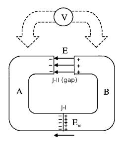
The actual experiment by Perminov and Nikulov has not been performed with the materials indicated in Figure 3. The authors used two equal tungsten electrodes (thus,  $\phi_A \simeq \phi_B$ ) and in any case they claim to have measured a current of the order of  $10^{-7}$  A (across a circuit resistance of 1 M $\Omega$ ). They also assert that such a current is not ascribable to Thomson or Seebeck effects.
