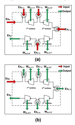
Figure 4. Exergy distribution of the four-stage radial turbine.
