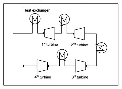
Figure 1. Schematic diagram of the four-stage radial turbine system.
