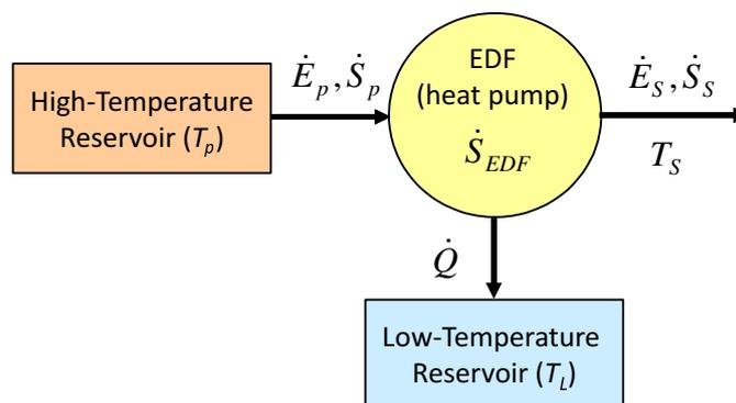
Thus, under the steady-state condition, we can write two basic balance equations for the EDFA model presented in Figure 3 according to the first and the second law of thermodynamics as follows:
