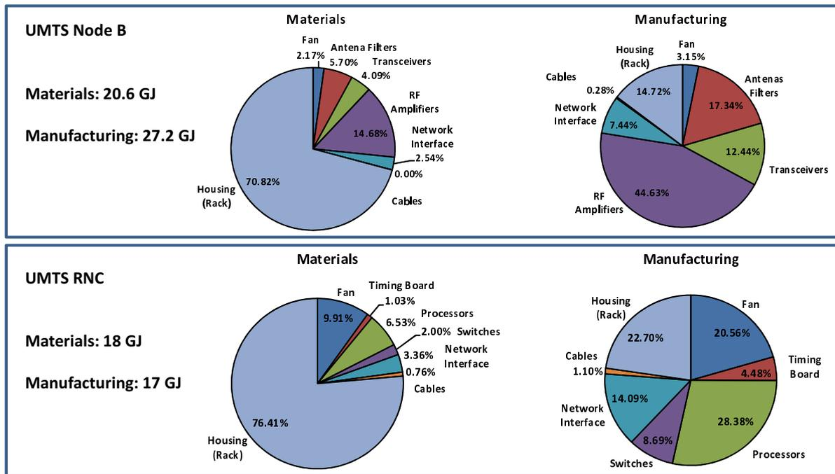
**Figure 9.** Exergy-based lifecycle assessment of the modeled UMTS radio access network for the City of Vienna [39,40]. The service life of network elements is assumed to be 10 years, while that of smartphones, two years.
