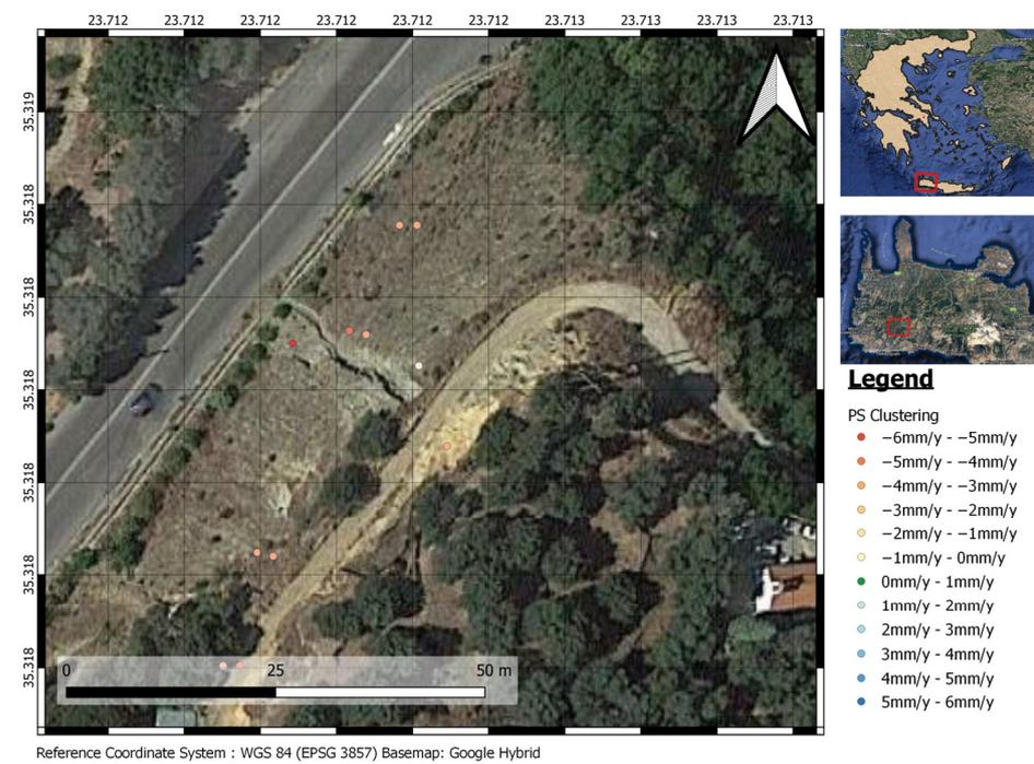
**Figure 2.** Identifying a landslide using P-PSI method and PS clustering focused on the specific region.
