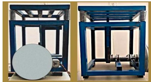
Figure 2. Final assembly of power generation system.
