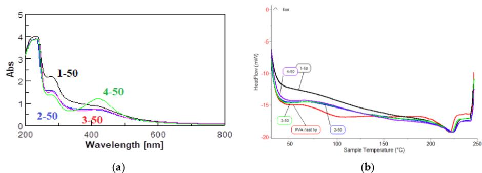
**Figure 1.** (a) UV-Vis spectra of batch 50 kGy; (b) DSC curves for the samples irradiated at 50 kGy.
