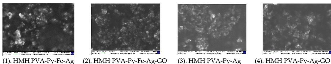
**Figure 2.** SEM images for hydrogel cross-linked with absorbed dose of 10 kGy.
