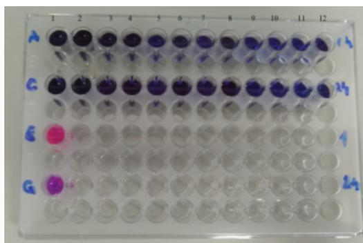
**Figure 3.** Qualitative testing of the antimicrobial effect of the HMH in the presence of resazurin.
