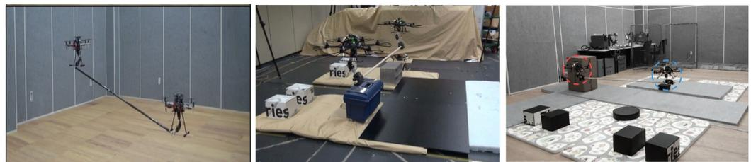
**Figure 3.** Cooperative Aerial Manipulation of a Rod with Multi-DOF Robotic Arms: [87,92,93] (from left to right).
