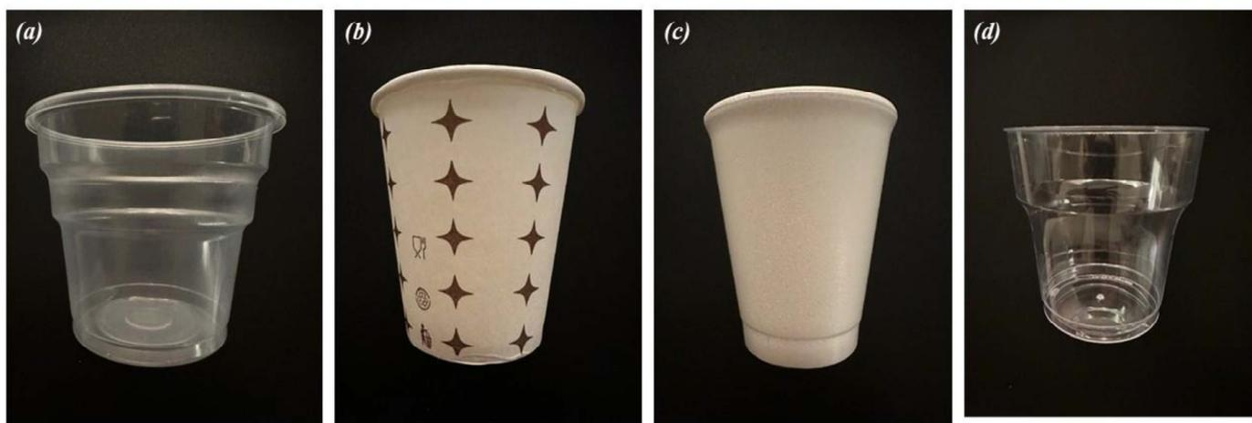
**Figure 1.** Plastic cups used (a) PP cup, (b) PE coated paper cup, (c) EPS cup (d) PS cup.
