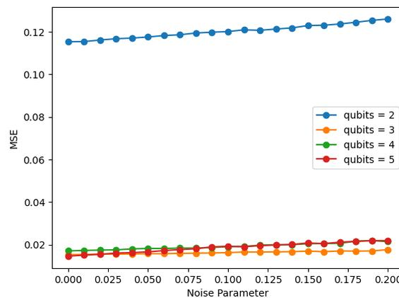
Figure 9. MSE from the traditional phase estimation algorithm for the 2/3/4/5-qubit datasets vs. noise.
