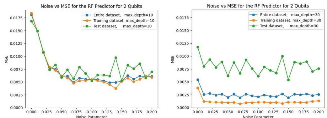
**Figure 6.** Overfitting example for the random forest algorithm and the 2-qubit datasets for a maximum depth parameter of 10 (left) and 30 (right). For these examples, the MSE of the training dataset (orange), test dataset (green) and entire dataset (blue) are presented for varying levels of noise.
