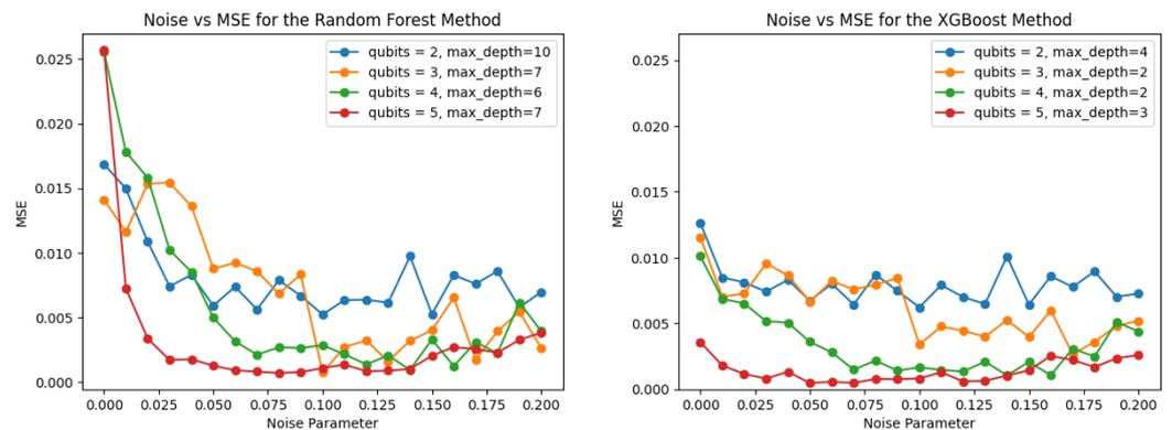
**Figure 11.** MSE vs. noise for all datasets when using the random forest (left) and XGBoost (right) tree-based algorithms. The legend of each panel identifies the dataset and value of max\_depth from Table 1 used to generate each curve.
