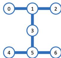
**Figure 8.** Device topology for the IBM Perth quantum computer [21]. The numbers 0–6 refer to individual transmon qubits.
