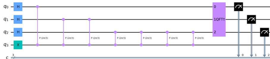
**Figure 1.** A circuit diagram for a 3-qubit QPE circuit where the unitary operator is a phase gate with phase  $2/3$ —this corresponds to a  $\theta = 1/3$  in the probability distribution.
