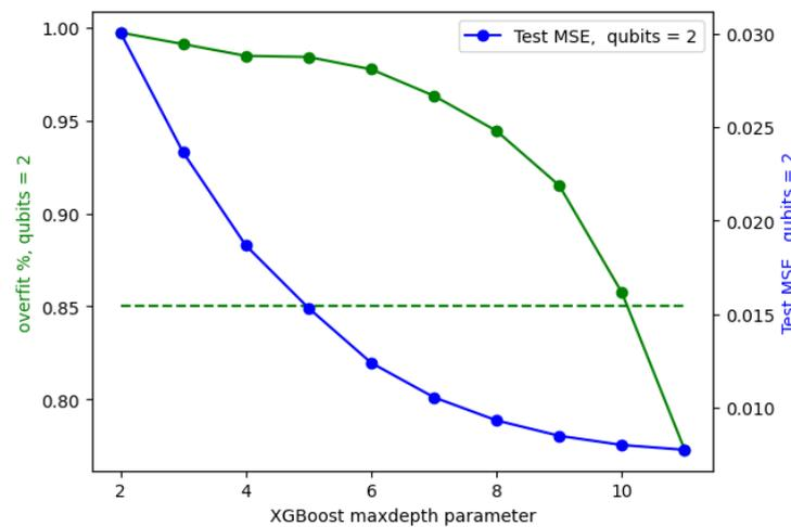
**Figure 7.** For the 2-qubit dataset, model MSE as measured on the test dataset (blue line, right axis), overfitting ratio (green line, left axis) and 15% overfitting threshold (dashed green line), for varying levels of the maximum depth parameter.
