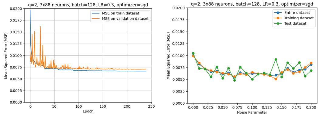
**Figure 12.** For the 2-qubit dataset, performance of the final NN model using the Ax-optimized set of hyperparameters as shown in Table 3. The training curves on the train dataset are shown in blue, and the validation split is shown in orange (left), and the model performance on the training/test/entire datasets are presented for varying levels of noise (right).
