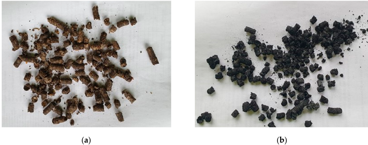
Figure 2. (a) D-PCS and (b) P-PCS (before and after the pyrolytic process, respectively).
