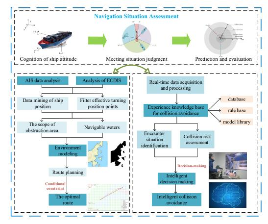
Figure 5. Ship intelligent decision-making technology diagram.
