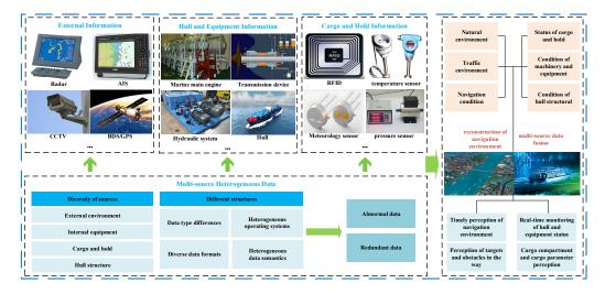
Figure 2. Ship intelligent perception technology diagram.
