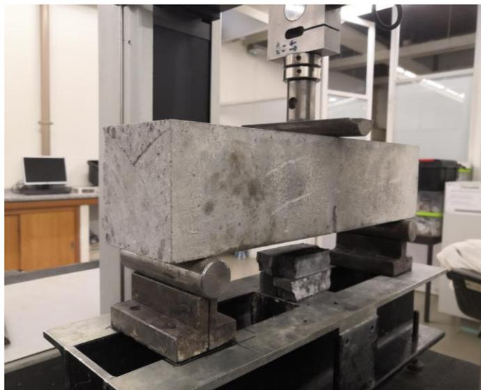
**Figure 8.** Demonstration of the flexural strength test.
