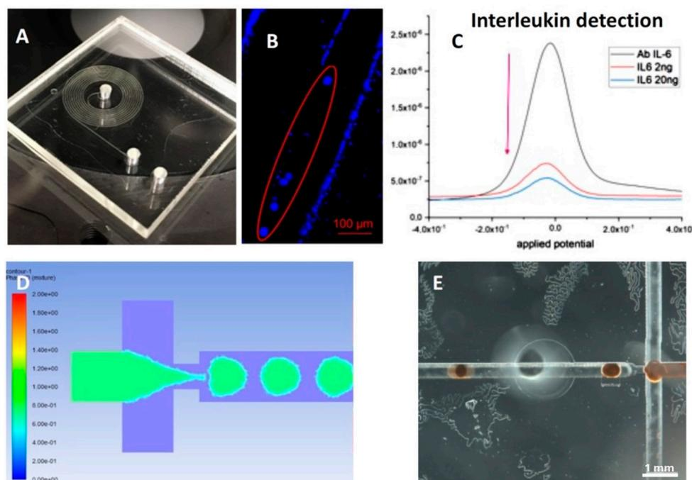
**Figure 2.** (A,B) Spiral channel for cell focusing. Red cycle highlight the position of cells in the channel (C) Interleukin detection by DPV. (D) Simulated device for droplets generation with emulsion of oil (green) in water (blue); (E) plastic device realized for droplet generation (red) in water.
