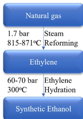
**Figure 5.** Production of synthetic ethanol from ethylene hydration.
