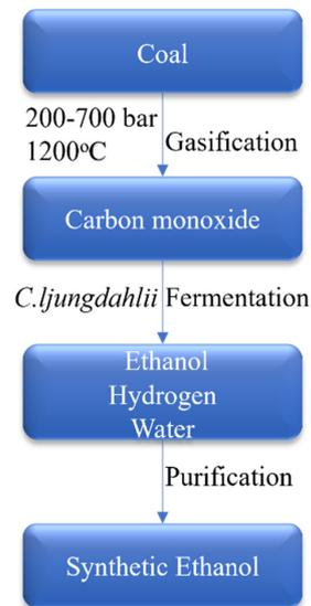
**Figure 3.** Production of synthetic ethanol from coal.
