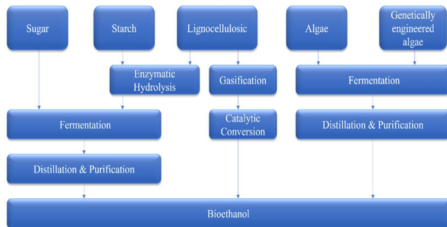
**Figure 6.** Bioethanol production from different generations of biomass.
