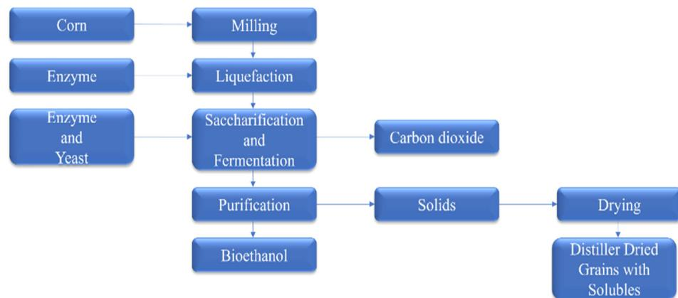
**Figure 7.** Dry-milling process.
