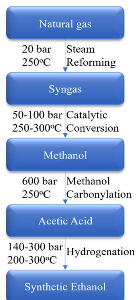
**Figure 4.** Production of synthetic ethanol from natural gas.
