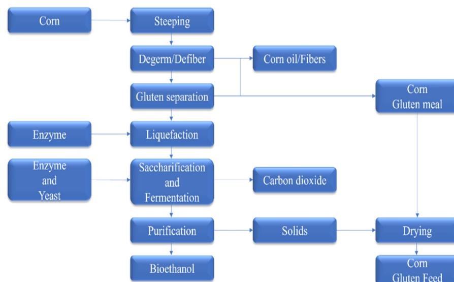
**Figure 8.** Wet-milling process.
