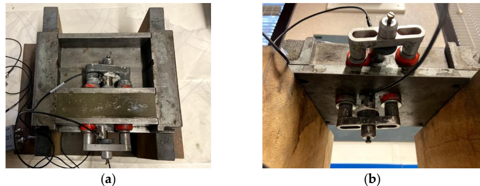
Figure 1. Acoustic emission setup: (a) top view showing two acoustical sensors and (b) side view revealing the bottom sensor.
