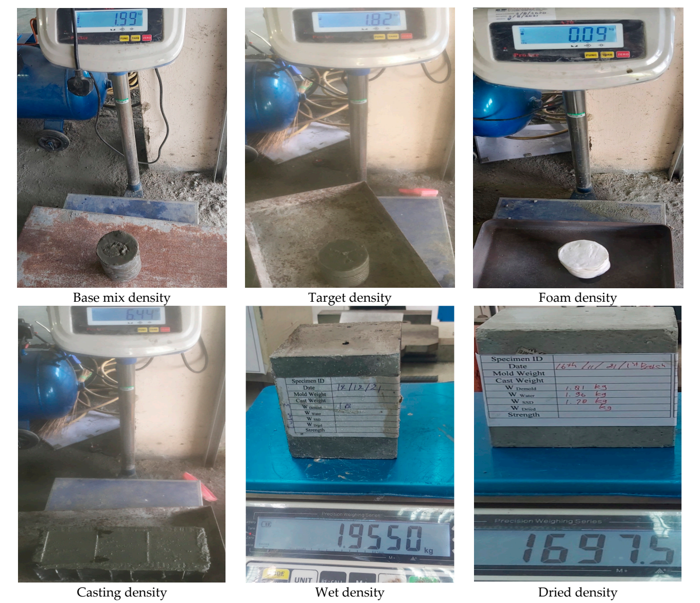
Figure 2. Fabrication of the foamed concrete and density checking of each stage.
