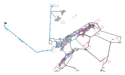
**Figure 1.** General layout of the underground mining exploitation (blue lines are the main airway tunnels and purple lines are the flexible ducts).
