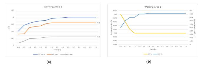
Figure 6. Results of a 7 h gas simulation at working area 1. (a) CO, NO and NO<sub>2</sub> in ppm; (b) O<sub>2</sub> and CO<sub>2</sub> expressed in percent.
