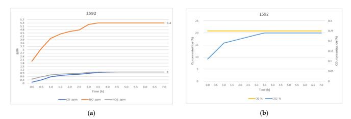
**Figure 7.** Results of a 7 h gas simulation at position  $\Sigma$ 592. (a) CO, NO and NO<sub>2</sub> in ppm; (b) O<sub>2</sub> and CO<sub>2</sub> expressed in percent.
