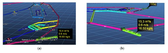
Figure 5. (a) Airflow velocity and quantity in working area 1. (b) Airflow velocity and quantity in working area 2.
