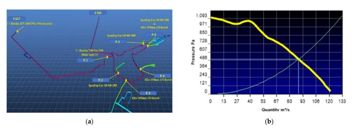
**Figure 2.** (a) Overview of the 3D ventilation model that was developed in Ventsim Design. (b) Operating point of ventilation system.
