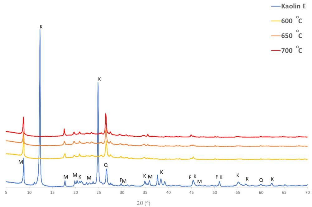
**Figure 1.** XRD patterns for Kaolin E and its calcined products in 600, 650 and 700 °C (K: Kaolinite M: Mica minerals F: Feldspar minerals Q: Quartz).
