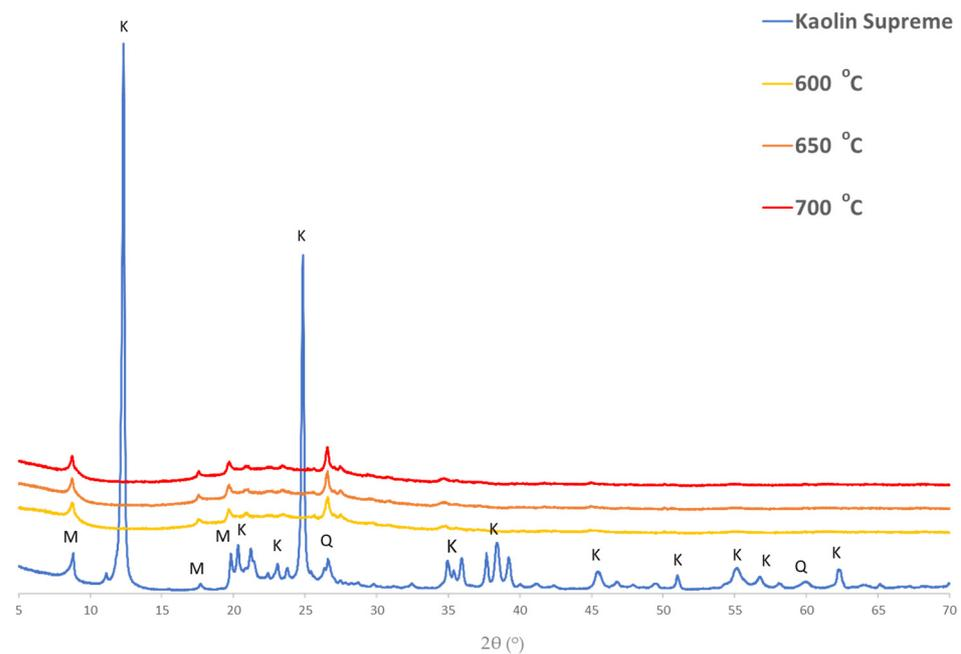
**Figure 4.** XRD patterns for Kaolin Supreme and its calcined products in 600, 650 and 700 °C (K: Kaolinite M: Mica minerals Q: Quartz).
