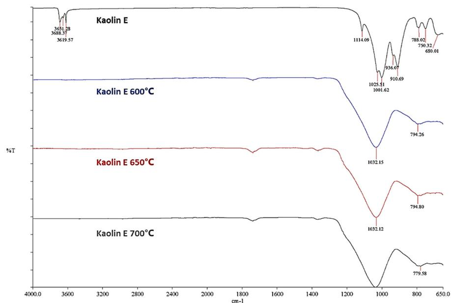
Figure 5. FTIR spectra of Kaolin E and its calcined products at 600, 650 and 700 °C.
