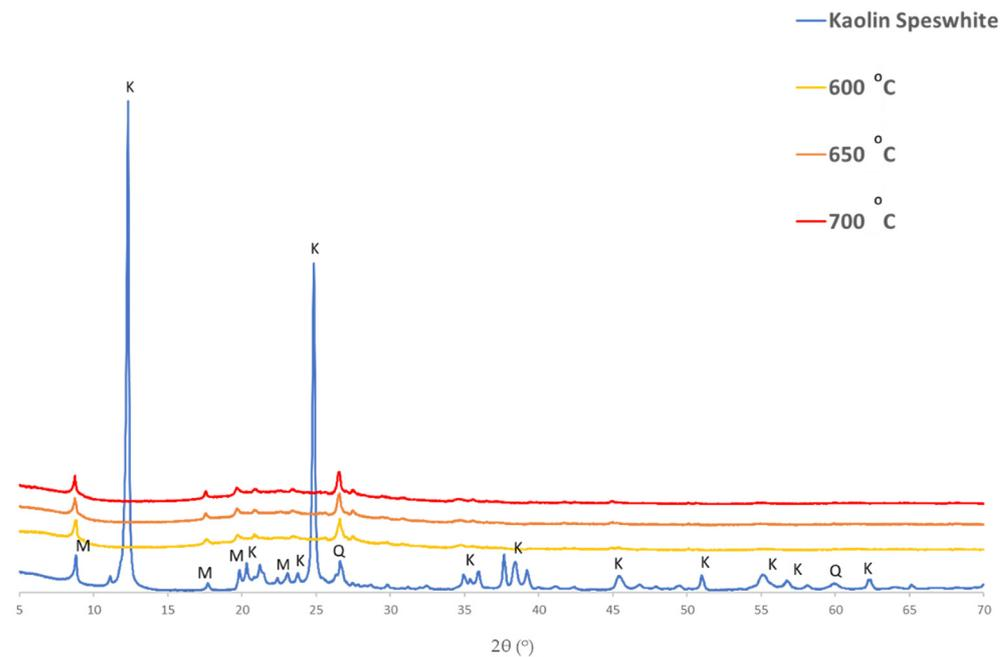
**Figure 3.** XRD patterns for Kaolin Speswhite and its calcined products in 600, 650 and 700 °C (K: Kaolinite M: Mica minerals Q: Quartz).
