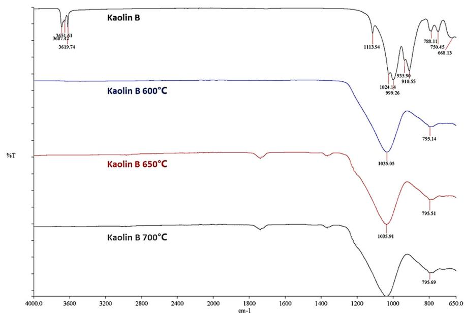
Figure 6. FTIR spectra of Kaolin B and its calcined products at 600, 650 and 700 °C.
