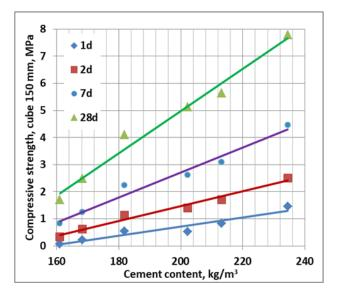
The strength of the applied pumice concrete depends on cement content, as in Figure 2.
