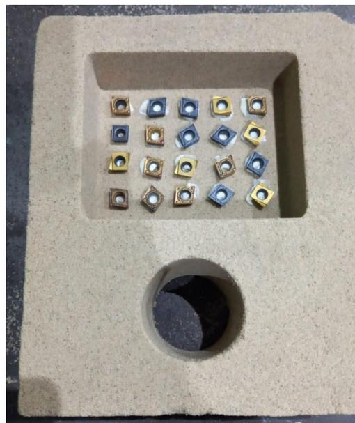
**Figure 1.** WC-Co tool tip scraps inserted into the mold cavity.
