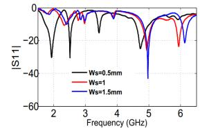
Figure 5. Return loss S11 of the proposed antenna for different widths (Ws) of the fractal slot.
