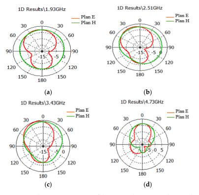
**Figure 9.** Radiation patterns in 2D of the proposed antenna on the two planes E and H plotted at the four resonant frequencies: (a) at 1.93 GHz, (b) at 2.51 GHz, (c) at 3.43 GHz and (d) at 4.73 GHz.
