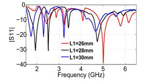
Figure 4. Return loss S11 of the proposed antenna for different lengths (Ls) of the fractal slot.
