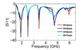
Figure 6. Variation of the return loss of the proposed antenna with different values of the height (H).
