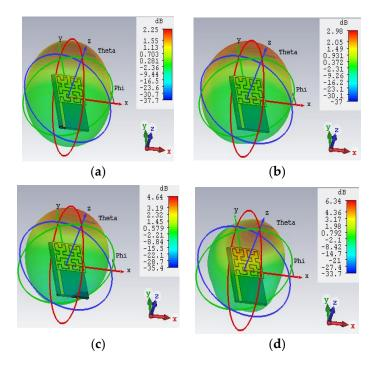
**Figure 10.** Three-dimensional radiation patterns of the proposed antenna at the four resonance frequencies: (a) at 1.93 GHz, (b) at 2.51 GHz, (c) at 3.43 GHz and (d) at 4.73 GHz.
