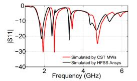
Figure 7. Return loss |S11| of the proposed antenna simulated under CST MWs and HFSS Ansys.
