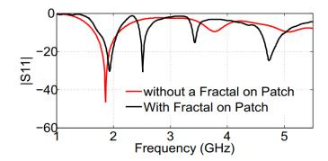
Figure 3. Return loss of the initial antenna and the proposed antenna.
