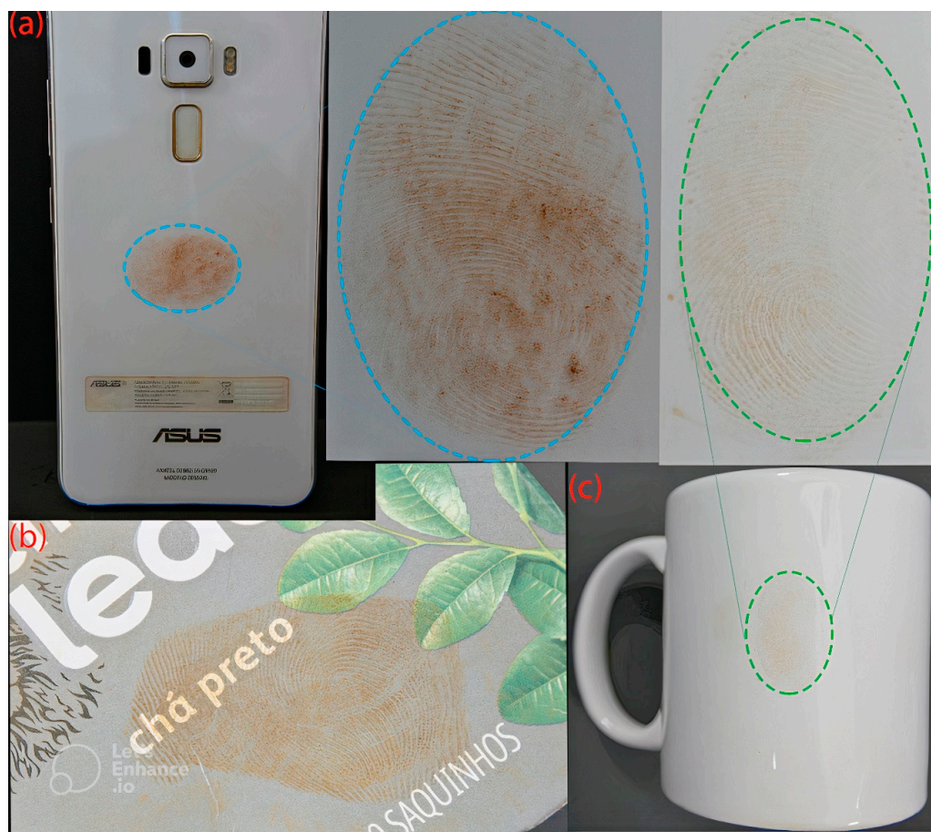
Figure 3. Fingerprints developed with RHL/chalcone on objects, such as (a) cell phone (glass); (b) box (cardboard); (c) mug (ceramic).
