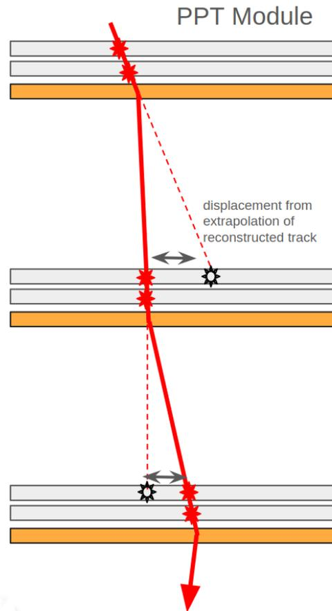
**Figure 3.** In this figure, a schematic of the working principle of the MSIS is shown. Three subsequent PPT modules are depicted. In red, the scattered track is shown with the hits on each silicon module (gray). The lead layers are drawn in orange. The three depicted modules allow for two independent displacement measurements. In a realistic detector, more modules would be present. To exploit the scattering induced by the last lead target, an extra silicon layer is needed.
