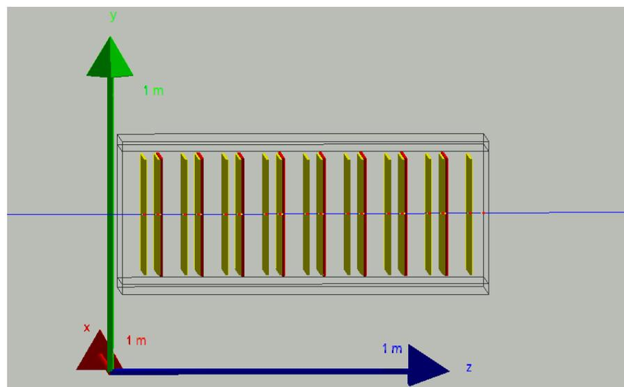
**Figure 4.** Graphical view of the GEANT4 simulation of the MSIS, with a simulated D event of generated energy 50 GeV/nucleon. Yellow volumes represent the tracking planes, while red volumes represent Pb targets. The blue track represents the trajectory of the particle and the red circles are hits on the detector materials. The three colored arrows indicate the reference frame used for the visualization, with the labels representing the dimension scale.
