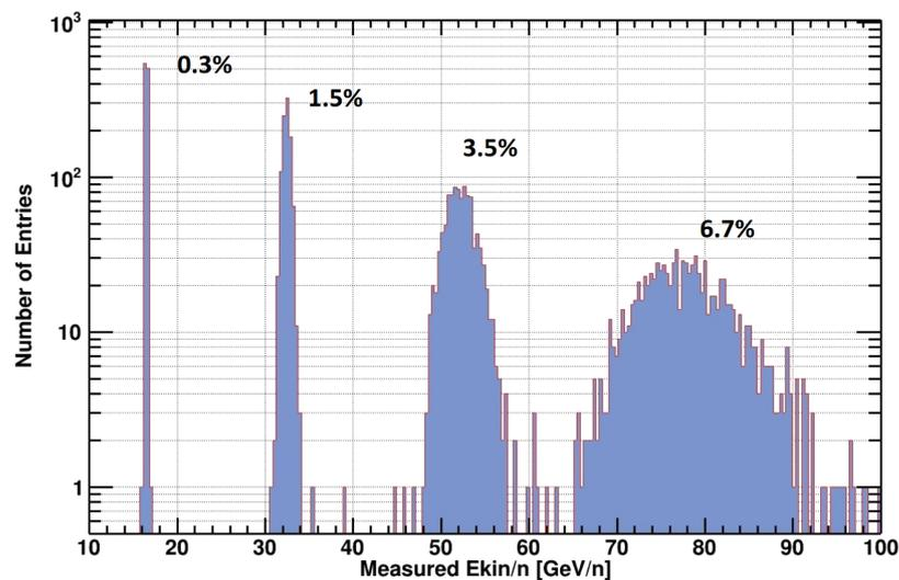
**Figure 2.** Performance of the proposed RICH design: reconstructed  $E_k/n$  for four monochromatic D beams of 16, 32, 52, and 80 GeV/nucleon. Measured resolution  $\sigma_{E_k}/E_k$  is also quoted close to each distribution.
