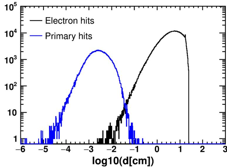
**Figure 5.** The blue line shows the distribution of calculated displacement between the interaction point of the primary particle on a given tracking layer and the extrapolated position of the primary trajectory, reconstructed with the previous PPT module. The black line shows the distribution of calculated displacement between the interaction points of the secondary electrons on the same tracking layer and the extrapolation of the primary trajectory measured in the previous PPT module.
