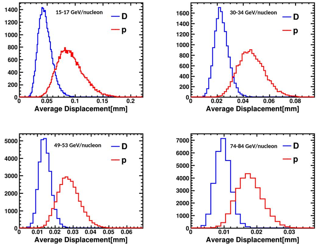
**Figure 6.** Distributions of average displacements measured in four simulated beams of D (blue) and p (red) in different  $E_k/A$  ranges by the MSIS. (**Top left**): 16–17 GeV/nucleon, (**top right**): 30–34 GeV/nucleon, (**bottom left**): 49–53 GeV/nucleon, (**bottom right**): 74–84 GeV/nucleon.
