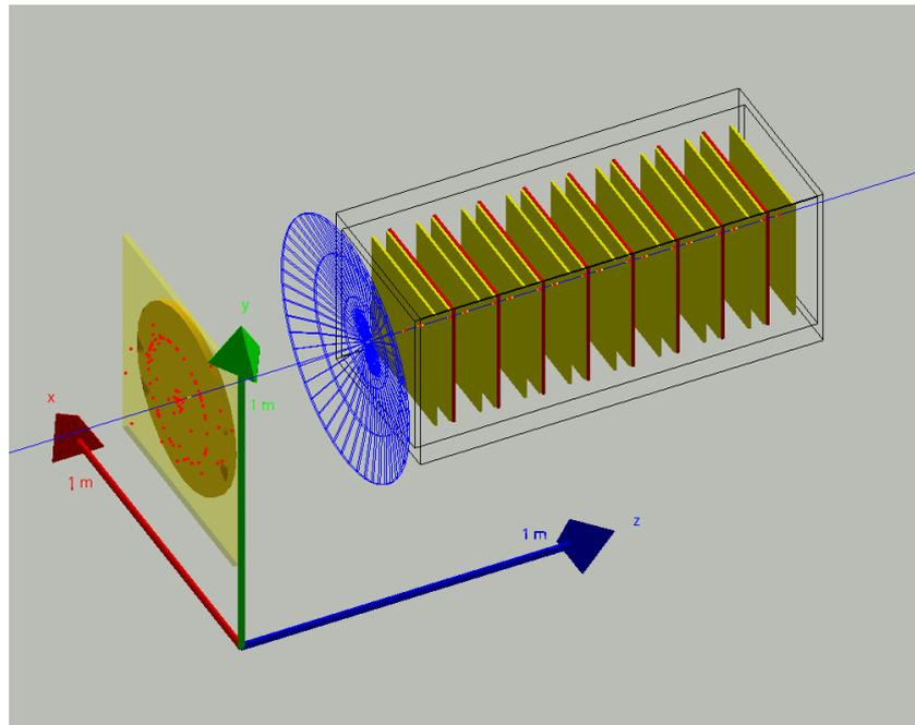
**Figure 8.** A GEANT4 simulation for a detector prototype. A deuterium nucleus is shot and traverses the entire the detector apparatus. In the figure, the blue line represents the trajectory of the primary particle, and the red dots are the energy deposits in the sensitive detectors. The three colored arrows indicate the reference frame used for the visualization, with the labels representing the dimension scale.
