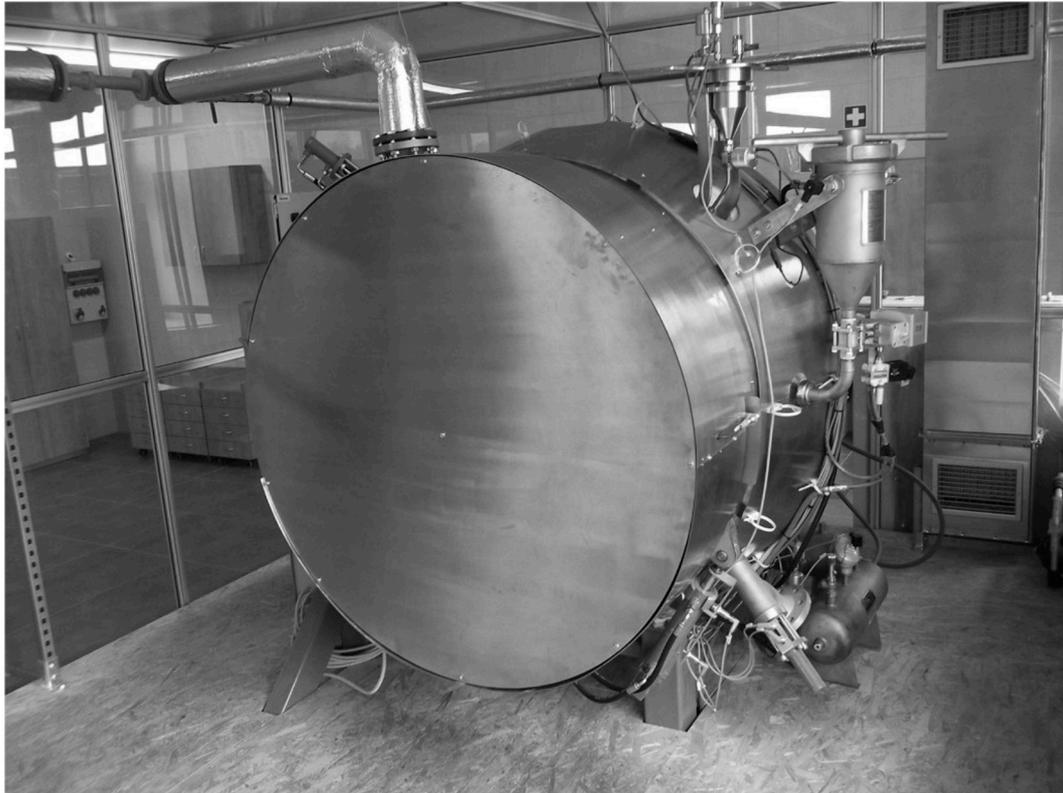
**Figure 2.** Illustrative picture of the explosion chamber CA 1M3 [21].
