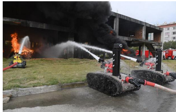
Figure 1. Firefighting robots approach the fire source and extinguish the fire instead of firefighters (Photo by reporter Zhou Weihai from Science and Technology Daily).
