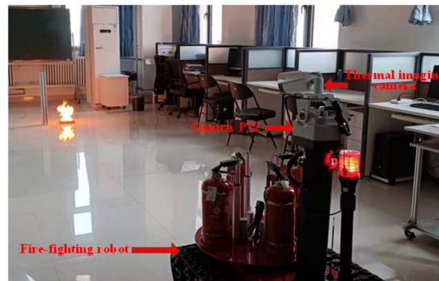
Figure 8. The firefighting robot collects thermal imaging flame images.
