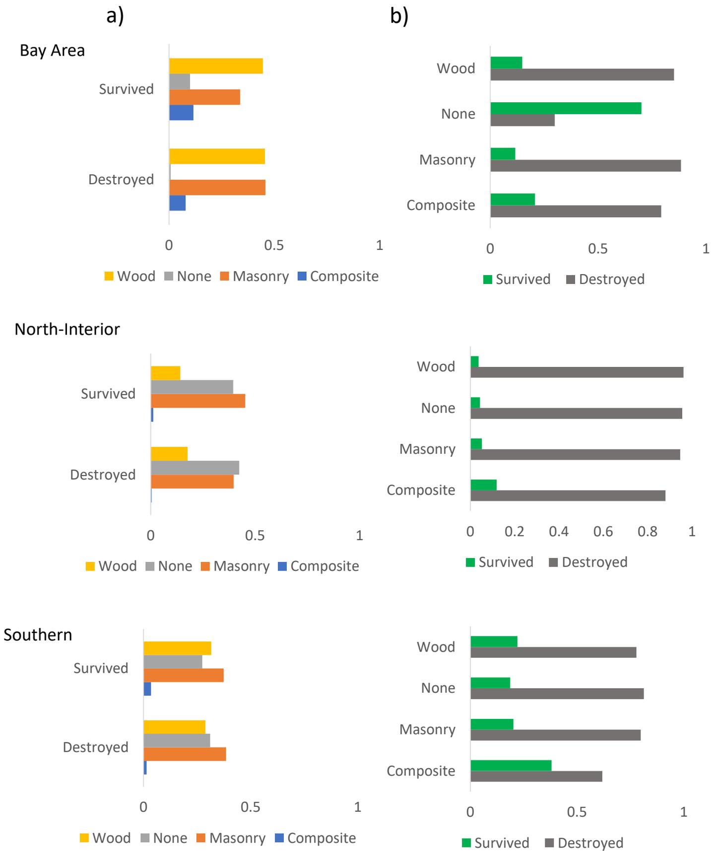
Figure S3: Proportion of deck material type for survived and destroyed structures (a) and proportion of survived and destroyed structures within deck material type classes (b) for three California regions.
