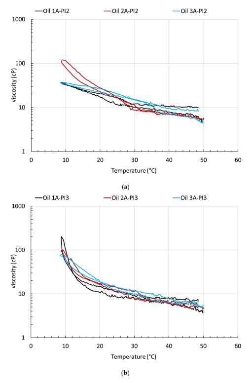
**Figure 9.** Viscosity as a function of the cooling/heating cycle 50 °C  $\rightarrow$  8 °C  $\rightarrow$  50 °C for oils (**a**) 1A-PI2, 2A-PI2, and 3A-PI2 and (**b**) 1A-PI3, 2A-PI3, and 3A-PI3, measured by applying a constant shear of 25 s<sup>-1</sup> and a cooling/heating rate of 1 °C/min.
