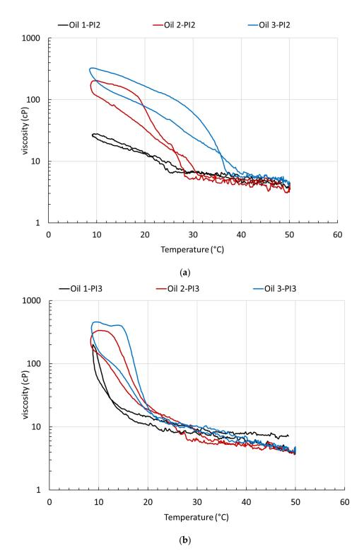
**Figure 5.** Viscosity as a function of the cooling/heating cycle 50 °C  $\rightarrow$  8 °C  $\rightarrow$  50 °C for oils (**a**) 1-PI2, 2-PI2, and 3-PI2 and (**b**) 1-PI3, 2-PI3, and 3-PI3, measured by applying a constant shear of 25 s<sup>-1</sup> and a cooling/heating rate of 1 °C/min.
