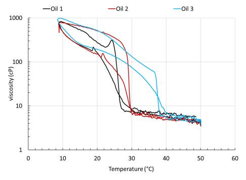
**Figure 3.** Viscosity as a function of the cooling/heating cycle 50 °C  $\rightarrow$  8 °C  $\rightarrow$  50 °C for oils 1, 2, and 3, measured by applying a constant shear of 25 s<sup>-1</sup> and a cooling/heating rate of 1 °C/min.
