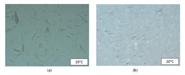
**Figure 2.** CPM images at 20 °C of oils (**a**) 2 and (**b**) 3. Wax crystals were not observed for oil 1 under the same conditions.
