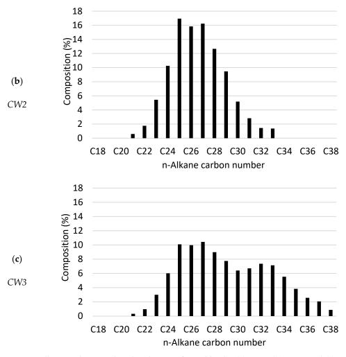
**Figure 1.** n-Alkane carbon number distribution of wax blends: (**a**) *CW1*, (**b**) *CW2*, and (**c**) *CW3* obtained by gas chromatography.
