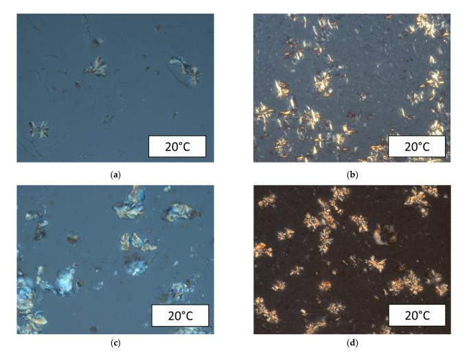
**Figure 4.** CPM images at 20 °C of oils (**a**) 2-PI2, (**b**) 3-PI2, (**c**) 2-PI3, and (**d**) 3-PI3. Wax crystals were not observed for oils 1-PI2 or 1-PI3 under the same conditions.
