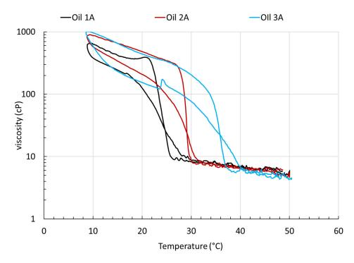
Figure 7. Viscosity as a function of the cooling/heating cycle 50  $^\circ$ C  $\rightarrow$  8  $^\circ$ C  $\rightarrow$  50  $^\circ$ C for oils 1A, 2A, and 3A, measured by applying a constant shear of  $25 \text{ s}^{-1}$  and a cooling/heating rate of 1 °C/min.
