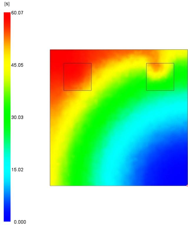
**Figure 9.** Resin injection from the bottom right corner of the mould, with the injection gate positioned at (24, 24), shown in Image 576 of the dataset.
