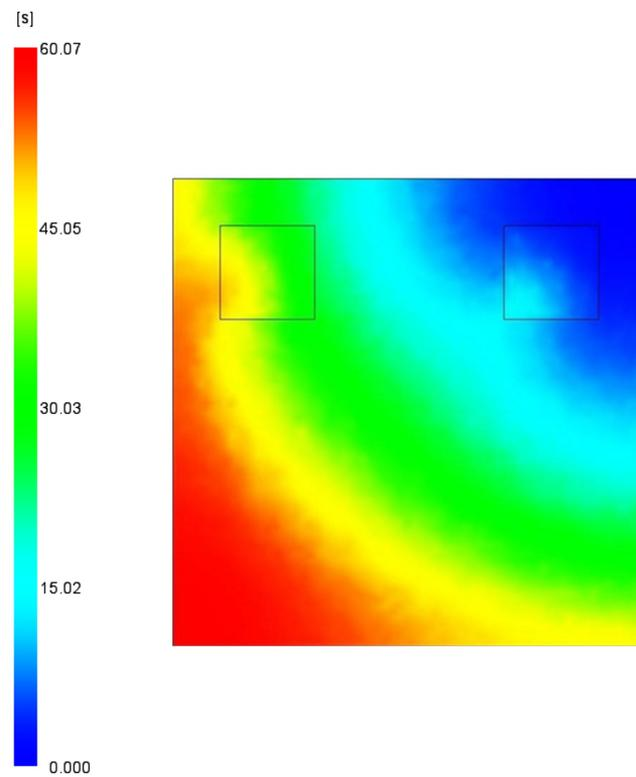
**Figure 7.** Resin injection from the top right corner of the mould, with the injection gate positioned at (24, 1), shown in Image 24 of the dataset.
