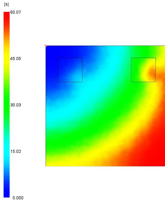
**Figure 6.** Resin injection from the top left corner of the mould, with the injection gate positioned at (1, 24), shown in Image 1 of the dataset.
