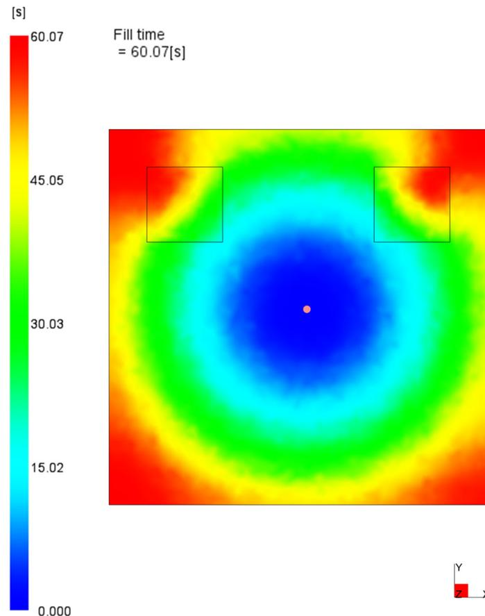
**Figure 5.** Example of a mould filling pattern and its time scale (central resin injection, Image 277).
