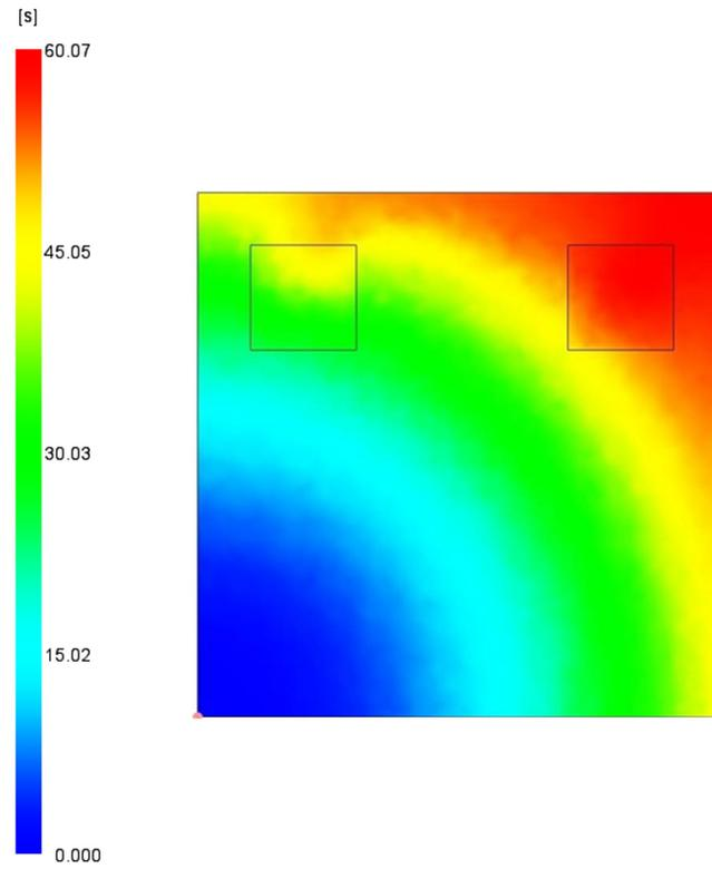
**Figure 8.** Resin injection from the bottom left corner of the mould, with the injection gate positioned at (1, 1), shown in Image 553 of the dataset.
