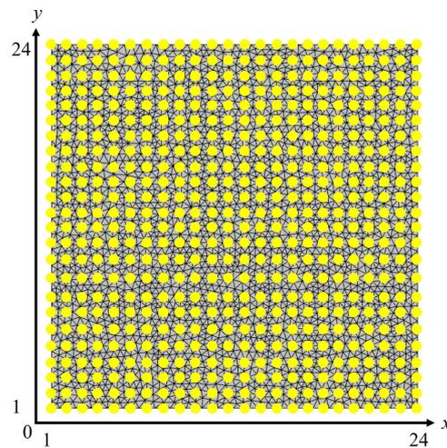
Figure 3. The 576 potential resin injection locations (yellow dots) on the mould surface projected on an (x, y) plane. (This image was previously published in [26]).
