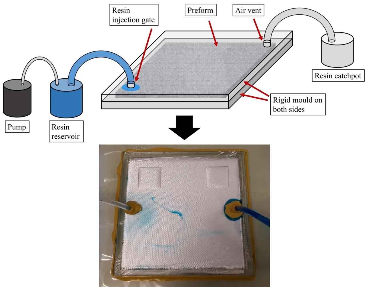
**Figure 4.** Schematic diagram of the experimental mould filling setup. Some stains are present on the exterior of the mould, due to mould reusing, which do not affect the process. (This image was previously published in [26]).
