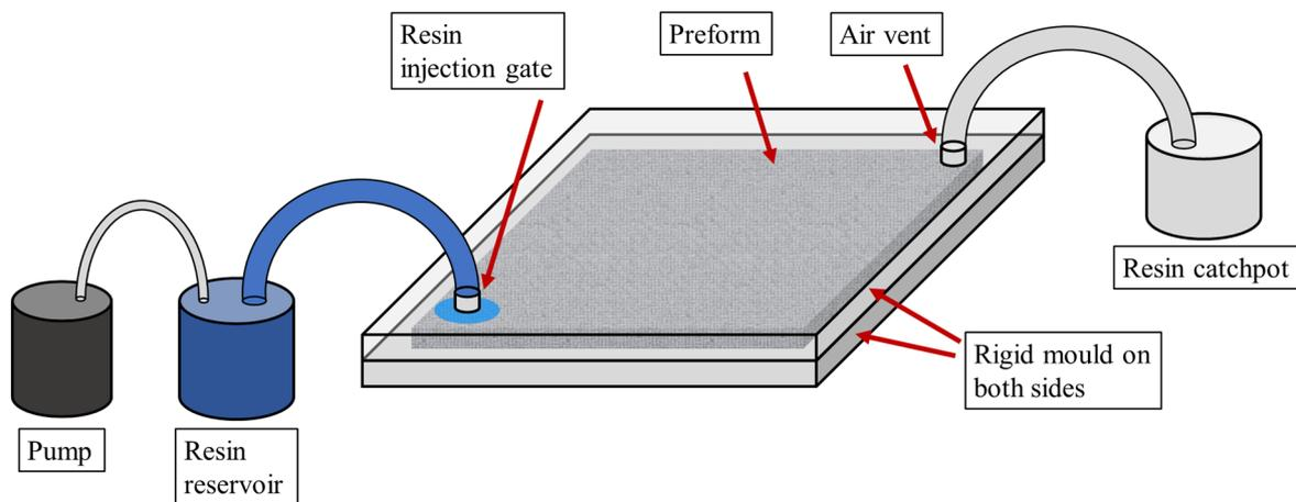
**Figure 1.** Schematic diagram depicting a typical composite mould filling process. (This image was previously published in [26]).
