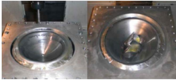
**Figure 19.** Mechanical failure on formed FML (reprinted with permission from [265]; copyright© 2021, Springer-Verlag France).
