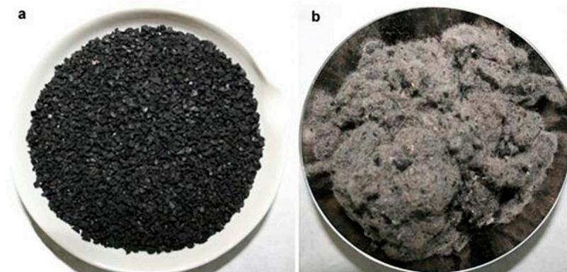
**Figure 4.** General aspects of the waste tire after shredding: (a) crumb rubber particles (1–10 mm) and (b) the reinforcing fibers (reproduced with permission from [54]).
