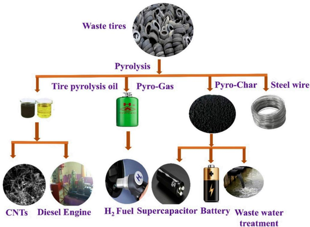
**Figure 3.** Waste tire pyrolysis products and their applications (reproduced with permission from [26]).
