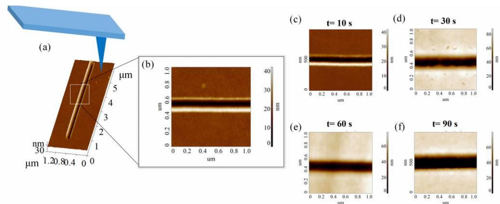
**Figure 1.** (a) P-AFL-patterned nanochannels; (b) details of PMMA pile-ups contouring the nanochannel; (c–f) effect of the pile-up removal for increasing times.
