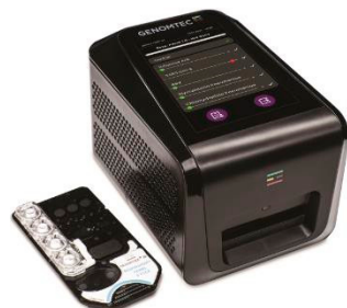
Figure 1. Overview of the analyser and microfluidics cartridge.
