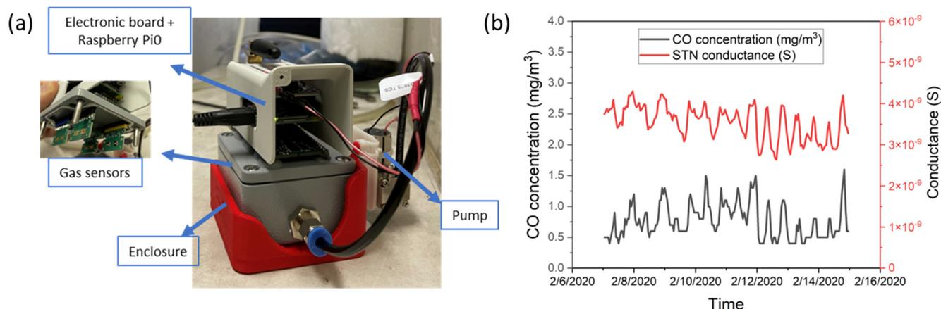
**Figure 1.** (a) Prototype of final sensor platform; (b) comparison between SnTiNbOx (STN) electrical conductance (orange line) and the real concentration of CO (EPA monitored, blue line), from 6 to 16 February 2020.
