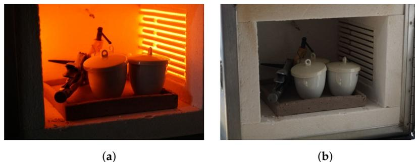
**Figure 2.** SMA annealing procedure. (a) Heating process using the muffle. (b) Passive dissipation of the crucibles.
