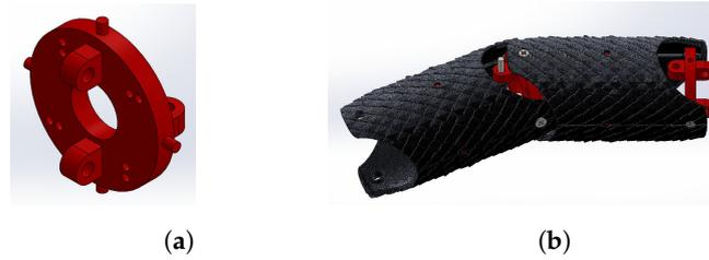
Figure 12. Rotational joint assembly. (a) Joint with anchorage. (b) Two links assembly.
